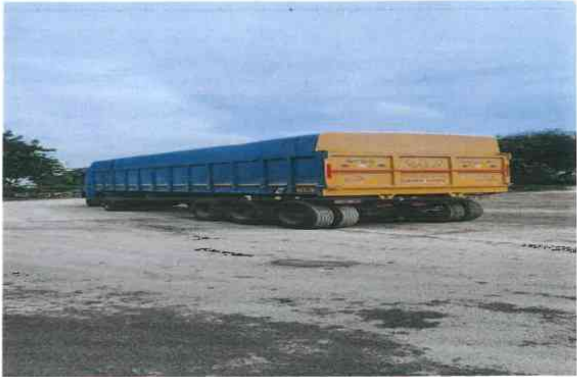
Ref 1: Transportation of Crushed material through trailer with closed body steel top
